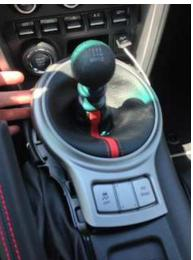
**3.** Using a flat head screwdriver, release the clip holding the traction control button harness into the bezel.Unscrew and remove the shift knob.
