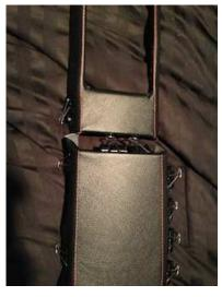
**13.** Begin gluing the fabric to the passenger side trim and hold in place with clips while it dries. Again, you may have to trim small pieces of fabric as you go to avoid folding and
