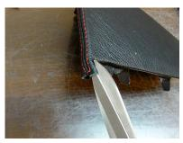
**18.** Let the glue settle and proceed with the front corners Đ make cuts along the seam to enable the seam to be folded under the hood.
