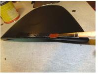
**3.** First glue the driver-facing edge of the hood - apply the glue along the edge with a brush - approx. 1-2cm to both sides of the edge.
