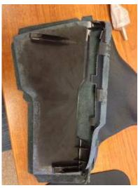
**5.** Carefully peel the stock vinyl from the plastic frame by lifting it up from the corners. The stock adhesive is not too strong and it should come off fairly easy without tearing.
