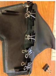
**8.** Use clips to hold the new boot down while the adhesive dries.
