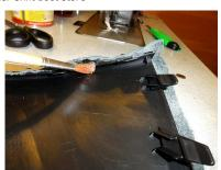
**6.** Then apply the glue to the bottom surface of the hood cover along the front edge, fold the leather and pres it strong to make it stick to the glue. Make sure the leather holds tight especially at the clips areas
