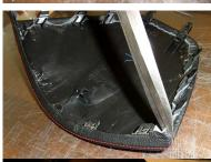
**20.** Once you are sure you cut enough, apply the glue to the bottom of the hood around the corners and fold the leather there. You should work with one corner at a time because you'll have to hole the leather folded with your fingers pressing it for some time until the glue settles. Then proceed to the other corner.
