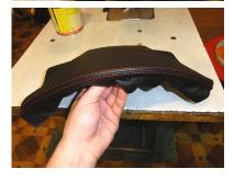
**5.** Make sure it's nice and tight, seam properly aligned to the edge and let the glue settle a bit.
