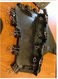
**9.** When the adhesive has dried, remove the clips.
