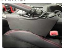
**3.** Lift the assembly up and slide the fabric up and over the brake handle. It will slip over it and the boot assembly will now be free.
