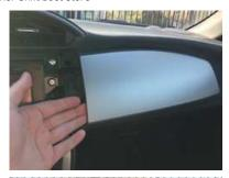
**4.** Line up the fabric for the stereo trim on the trim piece and clip it down in place.
