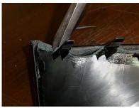
**16.** You will need to make small cuts in the leather on both sides of every clip to make it lay properly.
