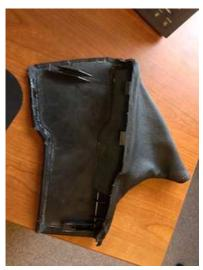
**10.** Inspect the boot to make sure all edges are properly secured. To reinstall into the car, reverse steps 1-3, slipping the new boot over the handle and pushing the clips down into place (this may require some added force with the leather option as it is now a bit thicker overall.)
